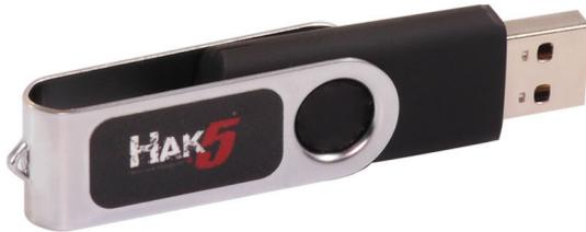
As can be seen, the unit looks like a USB flash drive one might obtain from any number of manufacturers but contains a programmable processor:
